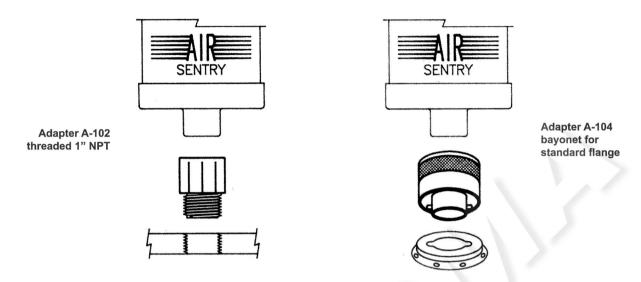
Air Sentry Breathers use a three-stage filtration design to ensure optimum protection by removing water vapor and solid contaminants before they enter the fluid system.
