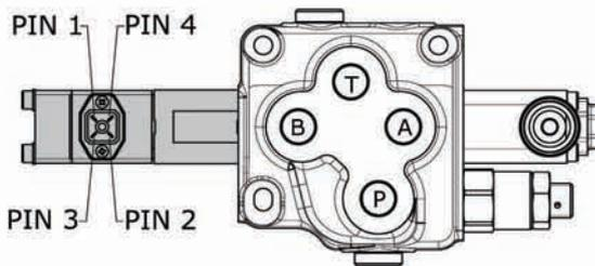
**CONTROL in A e B** = connect PIN 1 - 4 and 2 - 3
