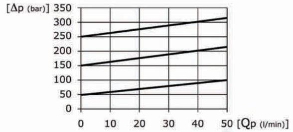
**Anticavitation valve curve**
