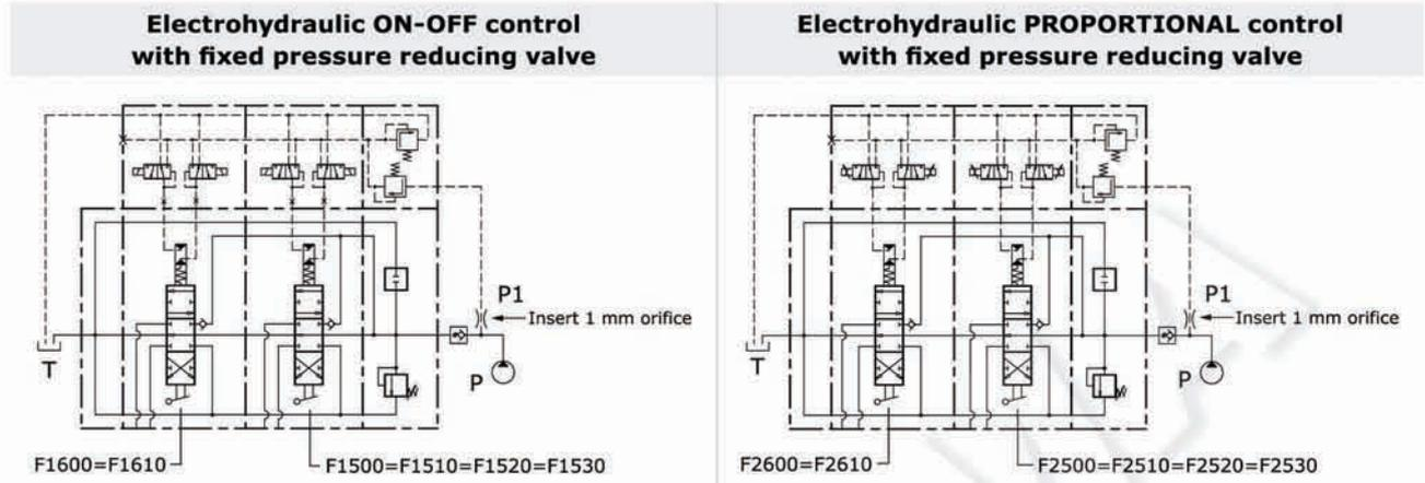
Proportional control kit, mechanically retrooperated, allows the maximum precision of positioning, limiting the hysteresis. The control is operated with PWM control of the current. PWM frequency suggest: 60-80 Hz
