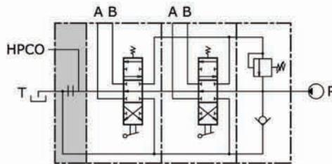
It is possible to transform monoblock valve from standard to HPCO version just by ordering the appropriate conic plug:
